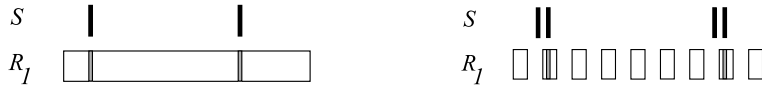
Figure 7.1: Instead of listening with 100 % duty cycle (left) as it is in the current implementation of politecast, duty cycling the listening and sending the packet twice within a time shorter than the sleep period (right) will lower the total utilization considerably. The duty cycles before could now be DC_S = 1\% and DC_{R_1} = 100\% and in the enhanced version DC_S = 2\% and DC_{R_1} = 50\% .
