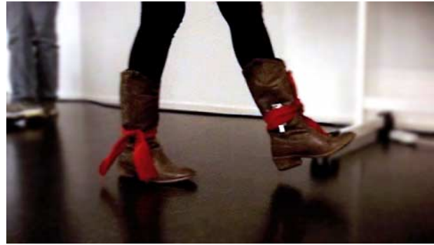
Figure 1. The walking artifact consisting of two sensor nodes attached closed to the feet tracking the rhythm of walking by measuring the radio signal strength between the two nodes communicating over radio.
